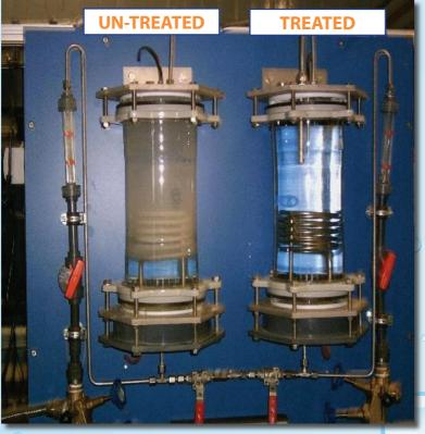
Nanosoft testing apparatus for scale prevention under DVGW W510 rules and Standards, Germany. Hard water is passing through the testing cells at a continuous flow where the water is heated at 80 degrees Celcius to raise the scale potential of the water even further. The test is designed to simulate the worst scenario with respect to water chemistry, this method simulates the water usage of the average German household over a lengthy time period. The pass rate for this Standard is 80%
